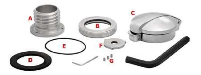
I. Place the large flat rubber gasket **D** under the adapter piece **A**. The thinner o-ring **E** goes between the ring adapter **B** and the Monza top cap **C**. Screw the assembly together.
