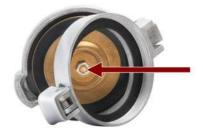
This lock nut holds the NMX002 top cap assembly together. Some adjustment of the nut is possible to alter the rate at which the cap springs open when in use. Check this nut is properly wound onto the bolt before proceeding further to ensure it doesn't fall off the thread into the tank.
