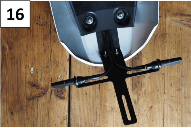
Mount the plastic mudguard with the aluminum mudguard in the same way as for disassembly.
