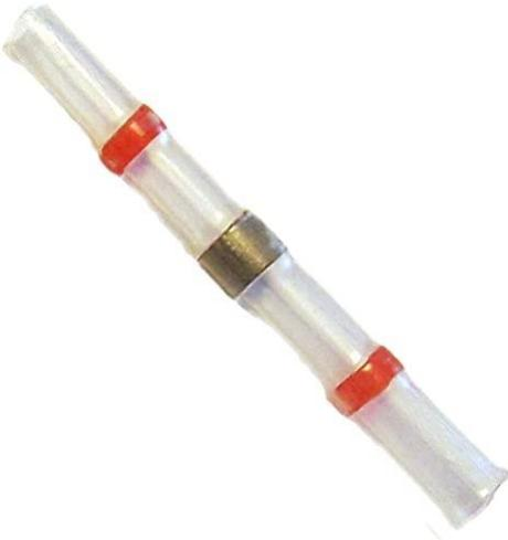
Connect both cable harnesses with the enclosed soldering connectors. To do this, push two cable ends into the soldering connector and heat it with a lighter or hot air dryer.
