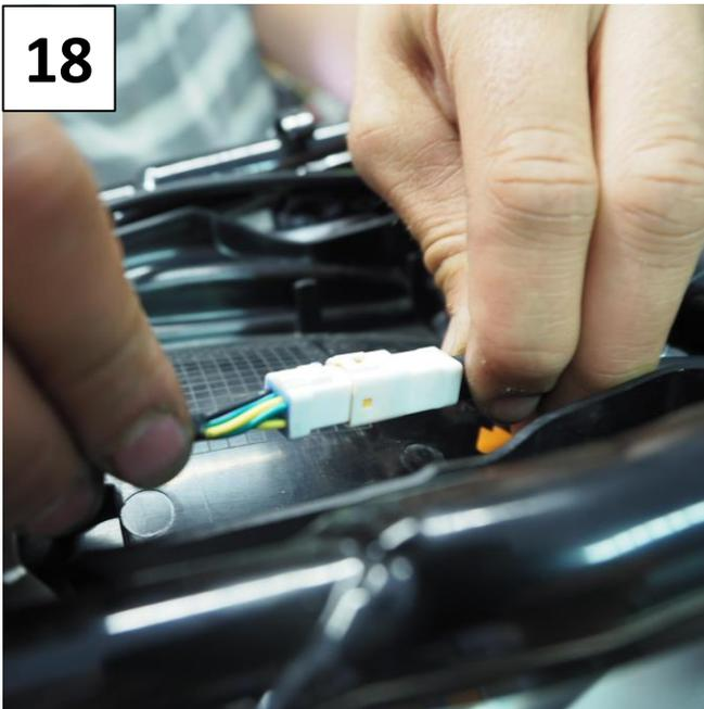
Reassemble the fender assembly with the motorcycle in the same way as disassembly.
