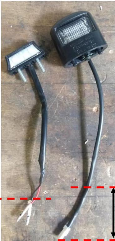
Cut the last 5cm of the wiring harness of the original license plate light. Cut off the connectors of the supplied license plate light and remove the last 5 mm of the insulation of the cable of the supplied license plate light and the cut cable of the original license plate light.
